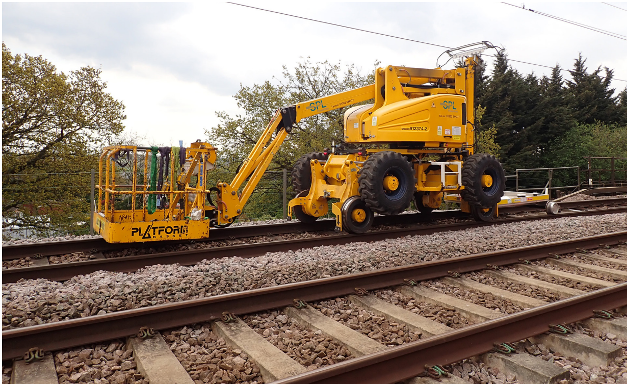
Figure 4: An example of a MEWP similar to that involved in the collision
