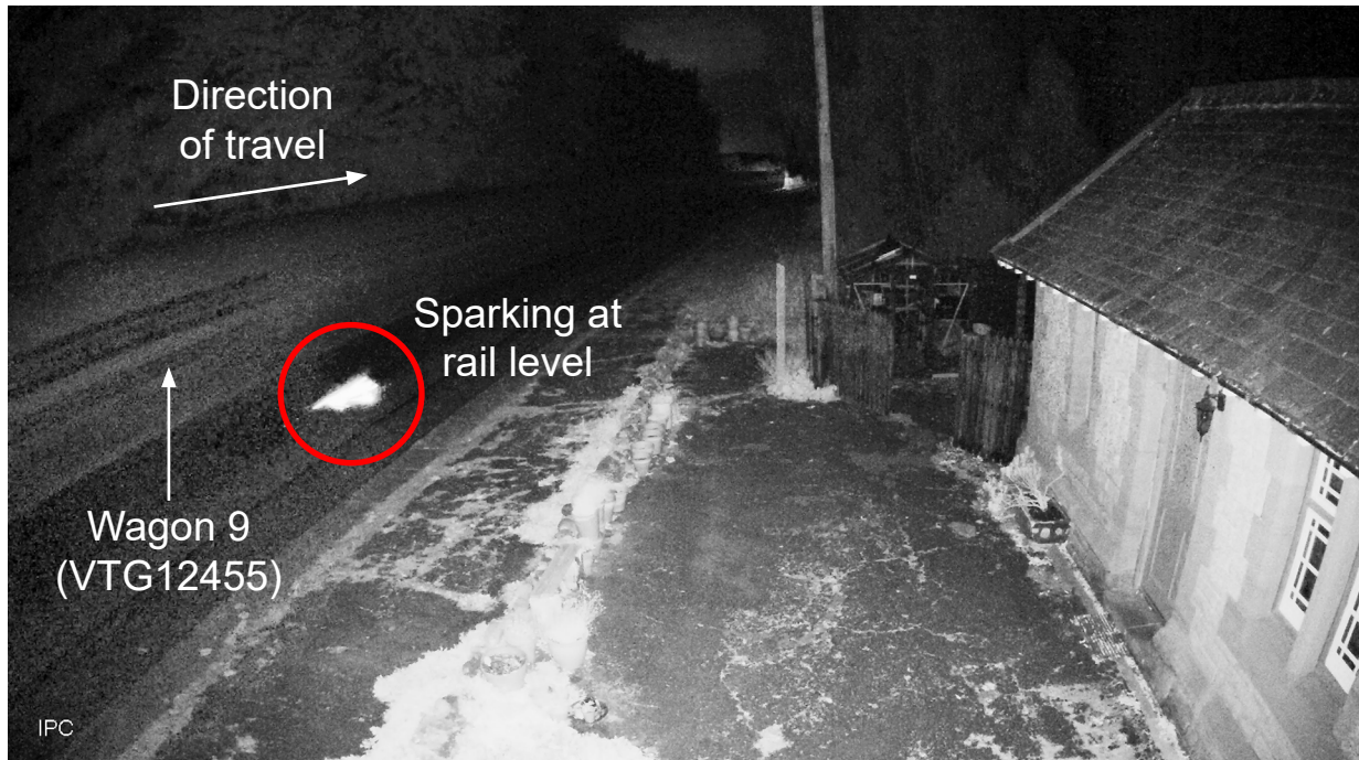
Figure 18: Sparking from the ninth wagon in train 6C00 at Little Salkeld (courtesy of Mike England).
