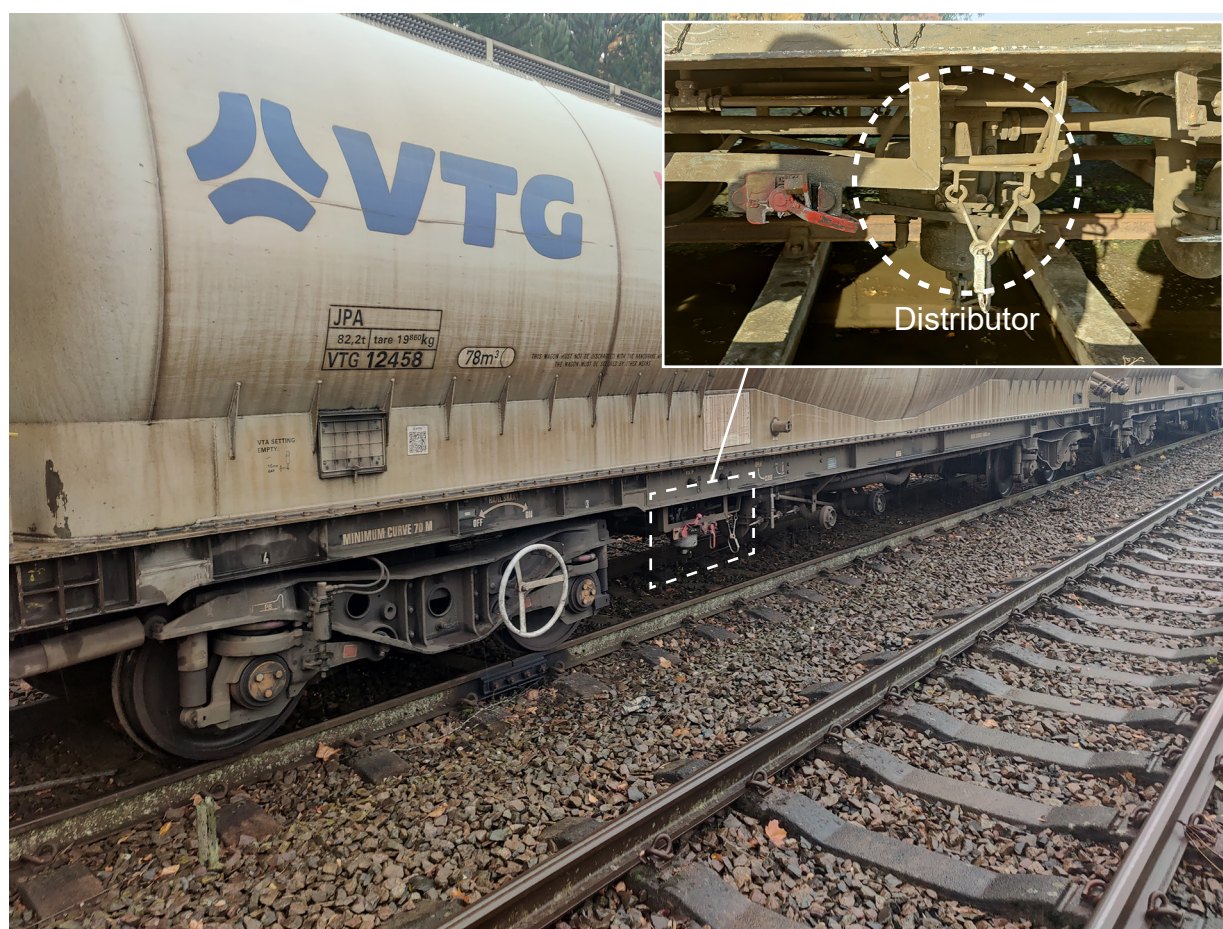
Figure 5: A JPA wagon and the location of its distributor (auxiliary reservoir hidden under wagon).
