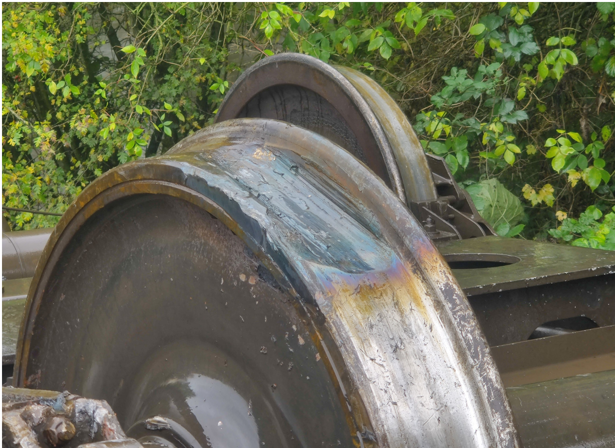
Figure 3: Wheel flat observed on the leading wheelset of the ninth wagon immediately after derailment.
