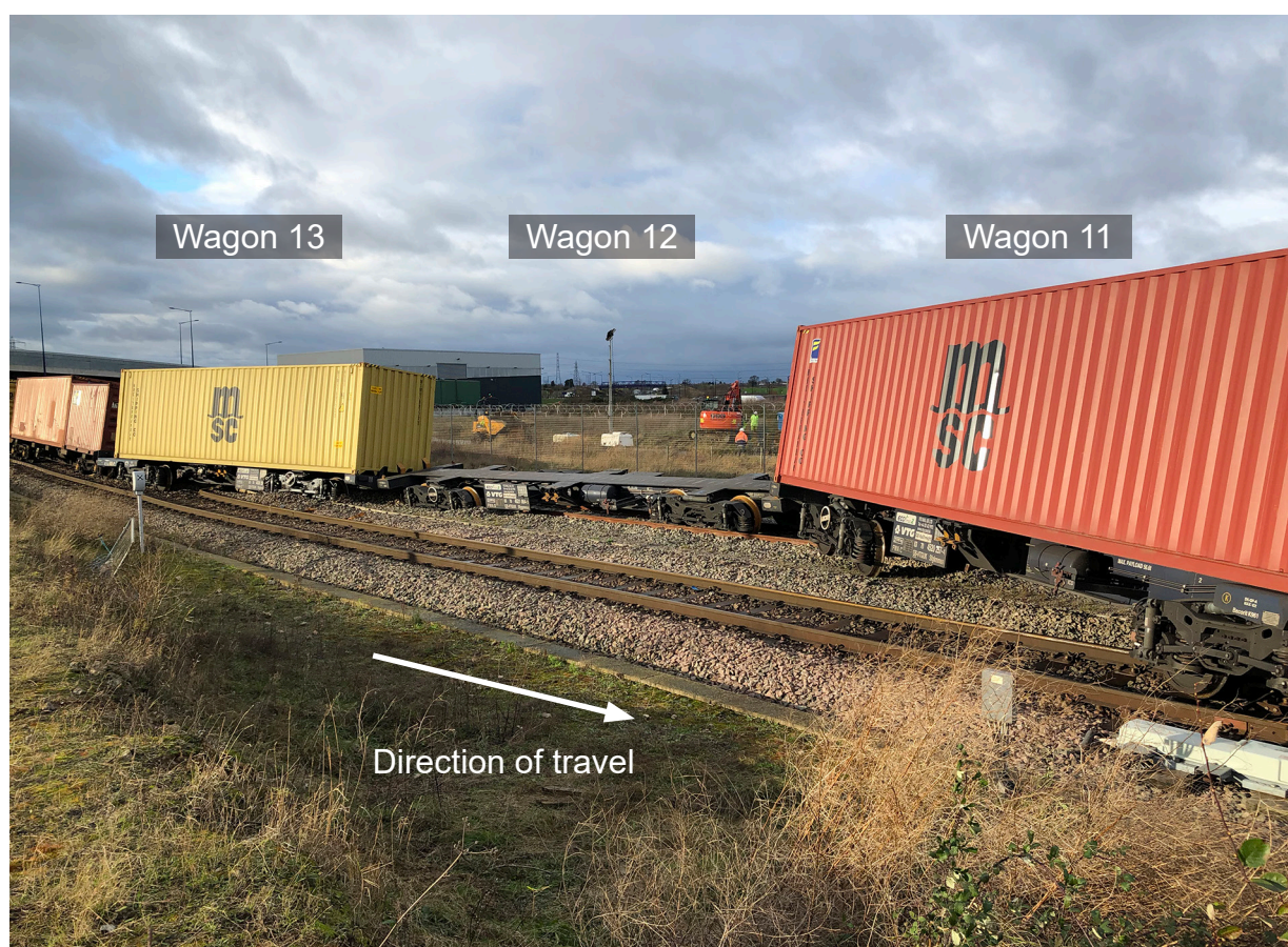
Figure 9: Final position of Wagons 11, 12 and 13 (photograph courtesy of VTG Rail).
