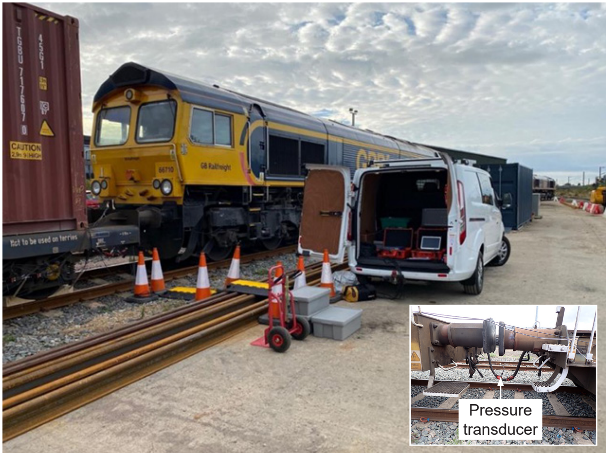
Figure B1: Brake testing arrangements. Inset shows pressure transducer fitted to a test point in the train brake pipe. (Main photograph courtesy Railway Braking Associates Limited).
